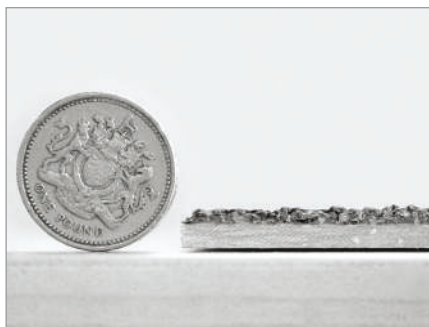
Coarse Grit particle size: 1.7mm
