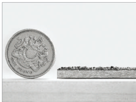
Medium Grit particle size: 1.0mm
