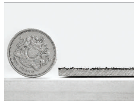
Fine Grit particle size: 0.5mm
